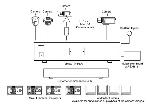
To use WJ-HD100 Series or a time-lapse VCR as a recorder, you need to install a Multiplexer board inside the matrix switcher.
