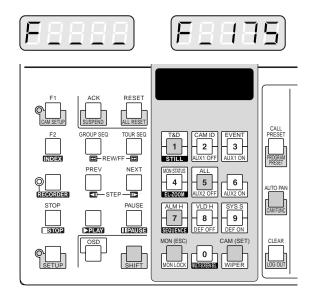
Press the numeric buttons to select an assigned function number, then press the CAM (SET) button.
