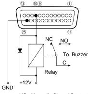
NC: Normally Closed Contact NO: Normally Open Contact
