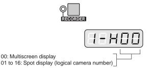
4. To exit from the recorder mode, select the camera. (Refer to p. 107 Camera Selection.) The indicator beside the button will go out. The monitor number and camera number will appear on the LED display again.
